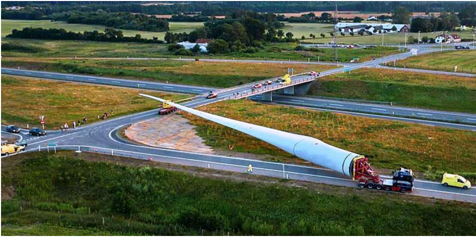
Fig. 4b. Transport of wind turbine blade
